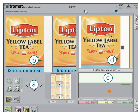
Main screen with print format preview (a), live image (b), roll map (c) and last defect image (d)
